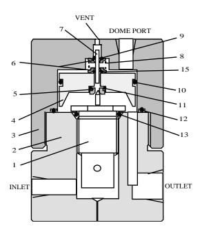
h. Lubricate cylinder walls of item 3 and seal 10 on piston then install piston 4 as shown
