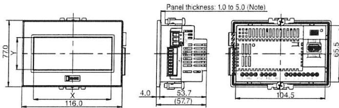
Transistor Output Model (FT1A-14KA-\* / FT1A-14SA-\*)
