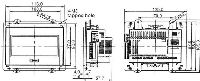
When using rear mount adapter (FT9Z-1A01)
