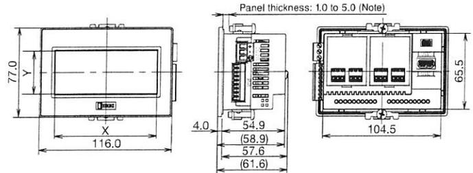
When using rear mount adapter (FT9Z-1A01)
