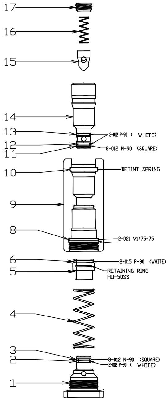
1. INSTALL #2 O-RING (ROUND) ON TO THE #1 BOLT
