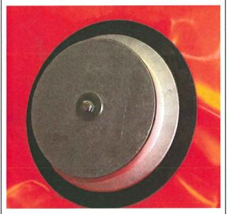
To identify the older version of the Jayco thief hatch plunger assembly: the lower washer (6") covers the whole vacuum gasket and the aluminum casting is smooth with no guides (shown above).
