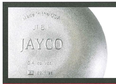
THE PURPOSE OF THE THIEF HATCH IS TO WORK IN TANDEM WITH THE VENT VALVE TO MINIMIZE THE ESCAPE OF LIGHT ENDS OF CRUDE IN LEASE STORAGE BY MAINTAINING A PRESSURE ON THE TANK. A VACUUM RELIEF FUNCTION IS ALSO STANDARD TO PREVENT A SUCTION OR DRAW DOWN FROM COLLAPSING THE TANK. THE THIEF HATCH PERMITS ACCESS TO THE CONTENTS OF THE TANK FOR SAMPLING AND GAUGING. THE VENT VALVE SHOULD BE SET TO VENT PRESSURE BEFORE THE THIEF HATCH.
