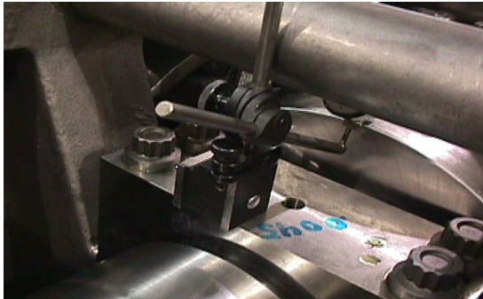
Dial Indicator Magnetic Stand Placement on Top of the Main Bearing Cap
