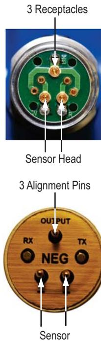
**Figure 26** Combustible (LEL) Sensor Assembly Alignment - 5.5V Cat-bead
