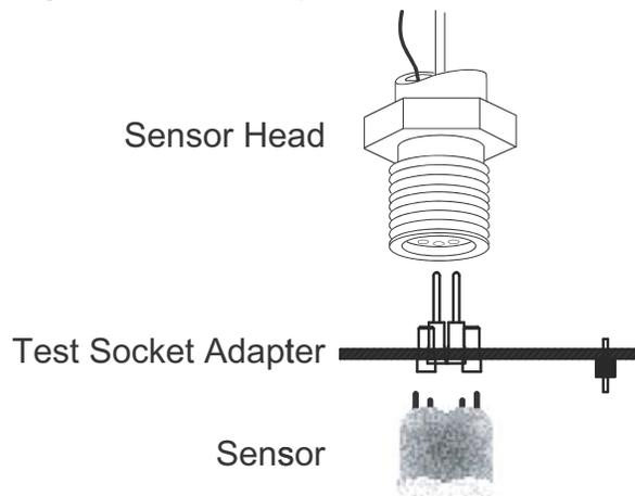
Measure the Voltage across the R (reference) and A (active) terminals on the Test Socket Adapter using a Digital Multimeter (DMM). See Figure 10.
