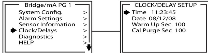
The device comes with a Clock & Calendar. The Time and Date must be set to correctly match its location. They are set at the factory in a 24 hour format but may require adjustment to match the location's time & date after shipment.
