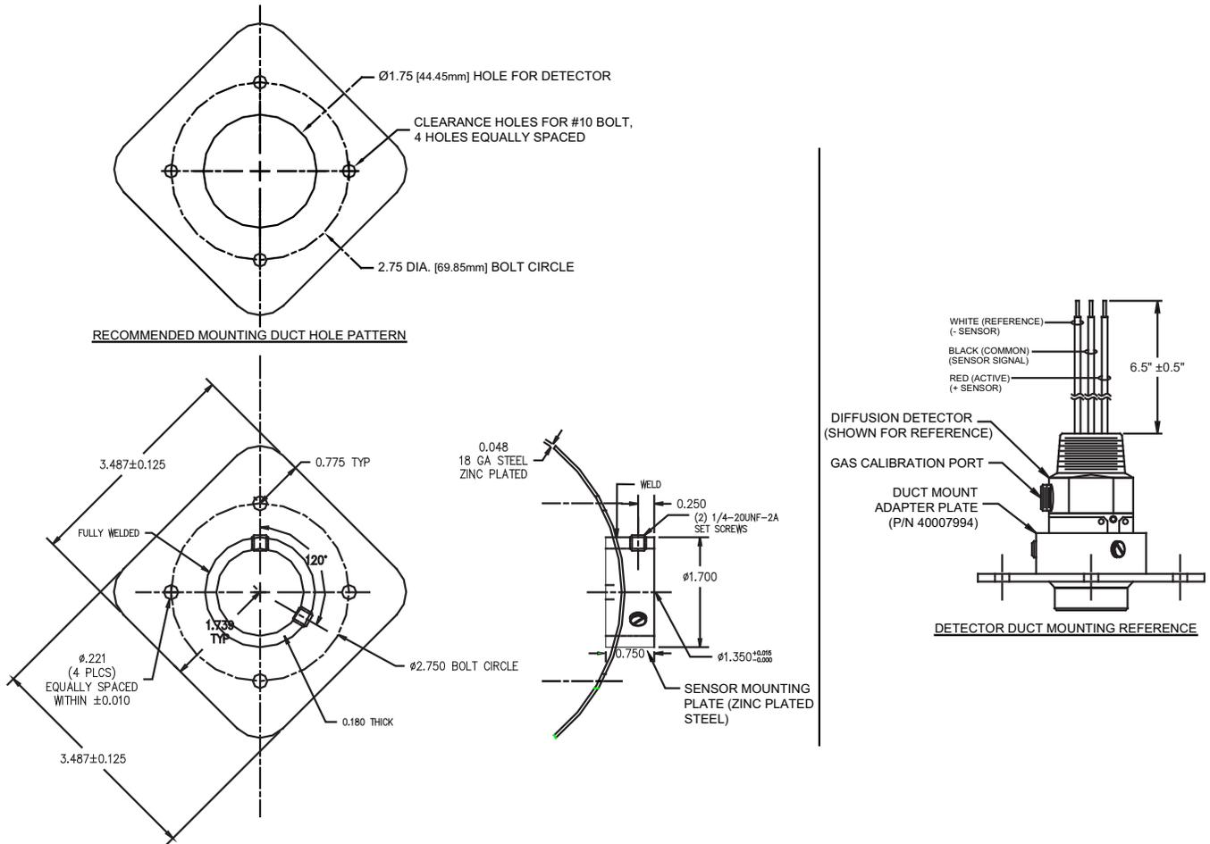
**Mounting a Toxic (E-Chem) Sensor Head Using a Duct Mount Adapter**
