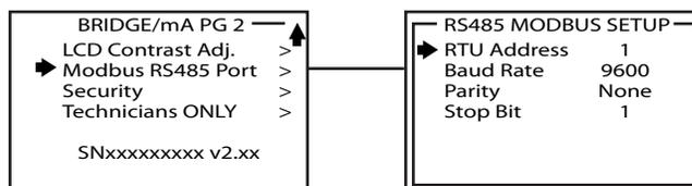
If the Relays/MODBUS RS-485 Option PCB is installed and the RS-485 port is in use, navigate to the MODBUS RS-485 Port display and assign each device its own RTU address, the legal range is 1 to 247.
