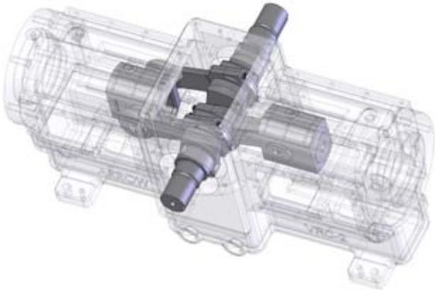
The Arrow VRC-2 can be packaged for single, two, three or four stage applications with double acting and steeple cylinder sizes from 2 1/4" to 8". Cylinders are air cooled which reduces packaging and maintenance costs. As a standard feature, cylinders have a variable volume clearance pocket for flexibility and adjustment to allow accurate fits for changing field conditions.
